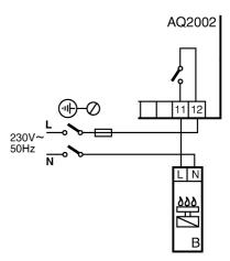
• ON/OFF boiler supplied by the line voltage and control by a free voltage contact
