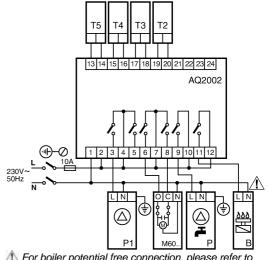
$\underline{\Lambda}$  For boiler potential free connection, please refer to boiler connection section
