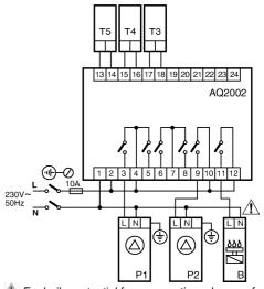
A For boiler potential free connection, please refer to boiler connection section
