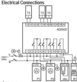
$\underline{\Lambda}$  For boiler potential free connection, please refer to boiler connection section
